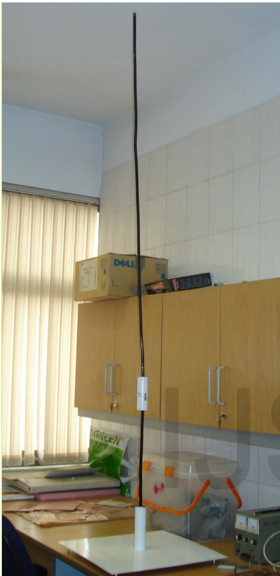
Figure 7. Photo of the fabricated antenna prototype
